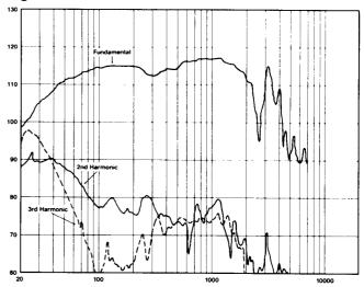
Figure 10 shows the fundamental, second harmonic, and third harmonic distortion of TAD 1601B low frequency transducer driven to produce a midband output of 115 dB-SPL at a distance of one meter. Input voltage 33 V.
