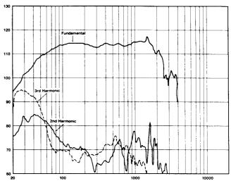
Figure 6 shows the fundamental, second harmonic, and third harmonic distortion of JBL 2226H low frequency transducer driven to produce a midband output of 115 dB-SPL at a distance of one meter. Input voltage 24 V.
