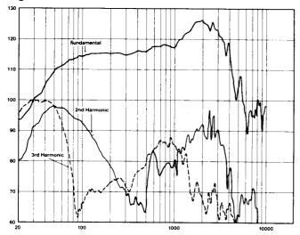
Figure 8 shows the fundamental, second harmonic, and third harmonic distortion of Electro-Voice DL15X low frequency transducer driven to produce a mid-band output of 115 dB-SPL at a distance of one meter. Input voltage 30 V.
