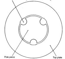
Figure 2 (B) Normal view of top plate, gap, and pole piece
