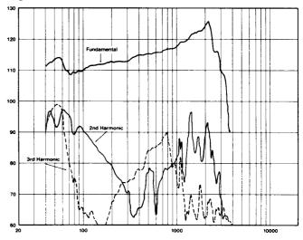
Figure 7 shows the fundamental, second harmonic, and third harmonic distortion of Electro-Voice DL15W driven with 40 volts. Measurement at one meter.
